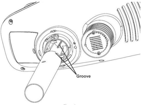
Reference Figure 4. Locate and align the groove on the sensor array and mounting pole.
