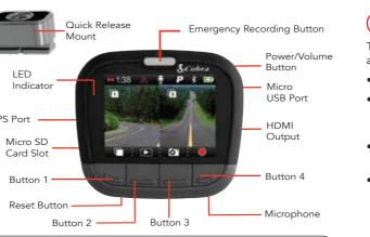
The functions of Buttons 1-4 are indicated by the icon directly above each button and change depending on the state of the unit.
