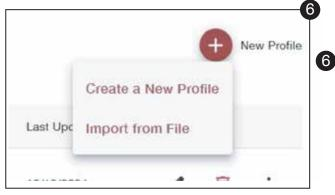
Select "New Profile" to set up a profile to save to your computer. "Import from File" allows you to select a profile currently saved on your computer. This profile can be one created by you or another user, emailed to you, or can be a custom frequency profile supplied by customer service. Your device does not need to be connected to create or edit profiles.
