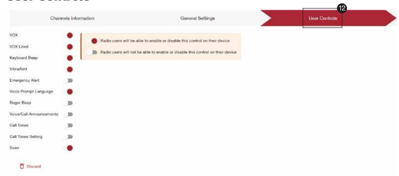
12 Turn the settings on or off in the device menu. If a setting is "ON" (toggled red) the setting/feature will be available on the device. If "OFF" (toggled gray) the setting will NOT show up on the radio menu. A user will need to reprogram via CPS in order to access the setting again from the device.
