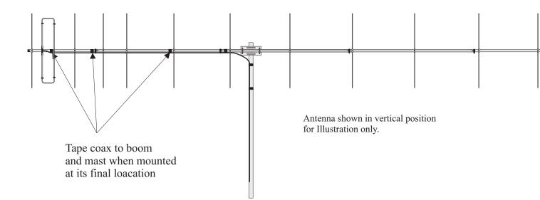
The antenna is now ready for mounting on your pole or tower. Route the coax along the boom and mast. Secure it using cable ties or electrical tape. Check the antenna over one last time to make sure everything is in place and secure. If you haven't already, Place the plastic end caps over the end of the booms.
