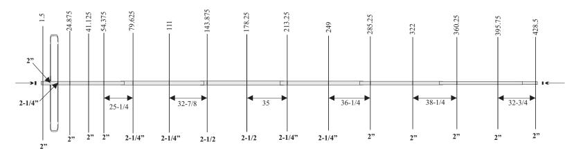
Once you have all the elements on in the correct location, check the alignment of the elements on the boom sections. Element locations are given on the top of the diagram above. You may use this to verify correct tube overlap between sections and that the booms are assembled correctly. Rotate the sections to align the elements if needed and re-tighen the clamps.
