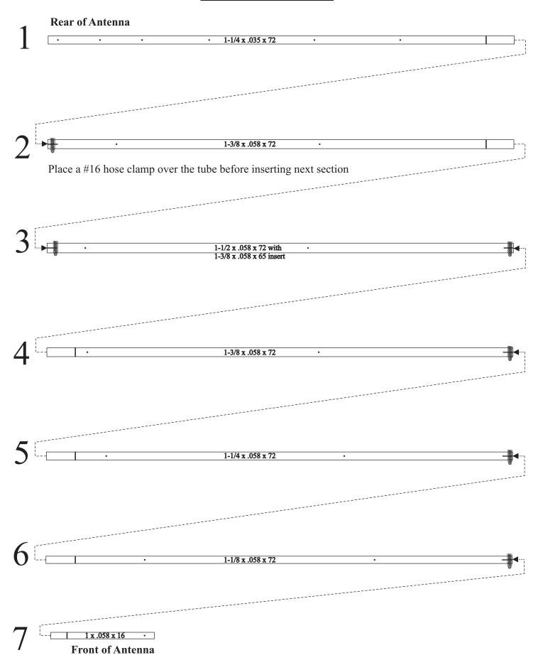
Insert each tube 3 inches into the next using the marks you made. Try your best to align the holes in each tube. Tighten the hose clamps just enough so that the tubes do not move. Final alignment of the tubes will likely be needed later. Now would be a good time to support the boom on a couple of saw horses or something similar.
