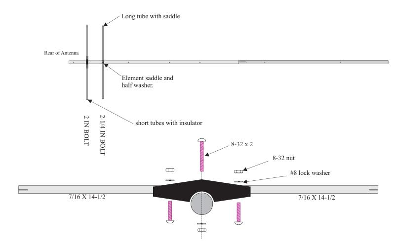
Mount the insulator on the Boom at the second hole from the rear of the antenna using the  $8-32 \times 2$  inch bolt. Attach the two short 7/16 tubes to the insulator using the  $8-32 \times 1$  inch bolt thru the holes in the ends of the tubes. Go ahead and tighten the nuts but do not crush the tubes.
