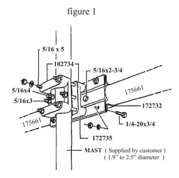
Note: If you use a galvanized 1-1/2 schedule 40 or 80 pipe as a mast, it has an O.D. of 1.9". You will need to put two split lockwashers under the 5/16 nuts on the four long bolts.
