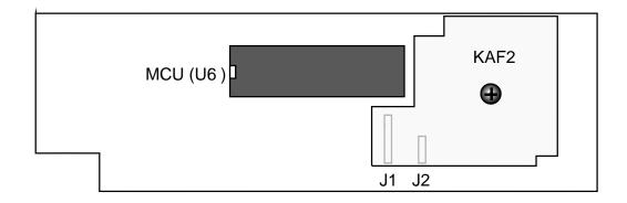
**1** If the standoff does not line up with the hole near the middle of the KAF2 module, you may have the pins of J1 and J2 shifted by one position.
