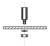
Plug the noise blanker module into J1 on the RF board, being careful to line up all pins of the connectors. Secure the module to the standoff using a 3/16'' (4.7 mm) screw and one internal-tooth lock washer.
