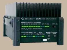
The KXPA100 is fully integrated with the KX2 and KX3 when used with the available adapter cable. The amp is automatically turned on whenever you set the radio's PWR control above 10 watts.
