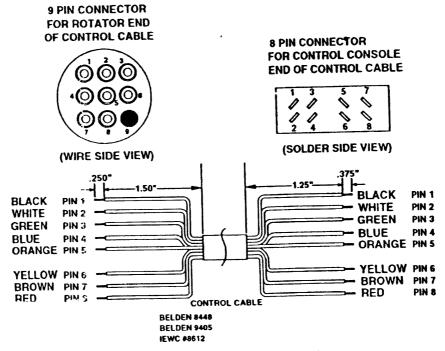
Figure 3 Control Cable Connector Attachment
