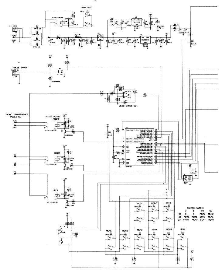
Figure 8 L DCU-3 Main PCB Schematic
