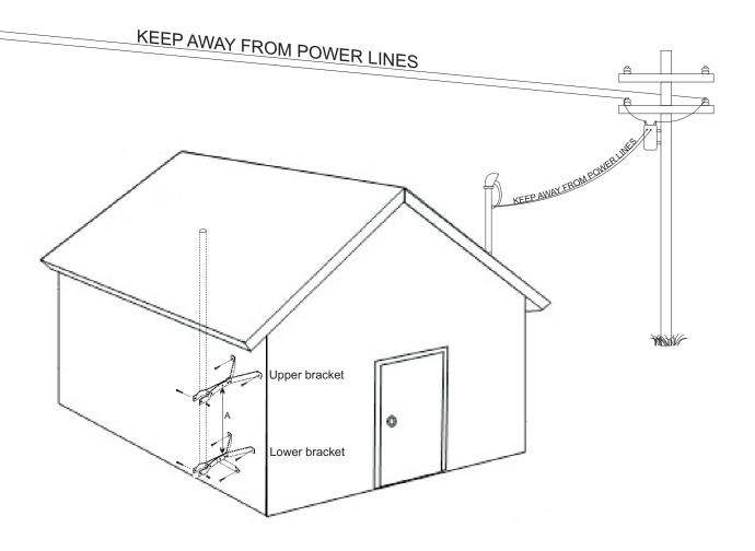
Choose a mounting location. The one shown is only one possibility. The highest point on the structure would offer the greatest final height of the antenna but access to the mounting location should also be considered. The mast may extend all the way to the ground if desired. This would add to the stability of the system and make grounding easier.
