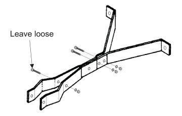
Assemble the top bracket as shown using two of the four arms, the supplied bolts, nut, and lock washers. Tighten the two closest bolts but leave the one closest to the V loose.
