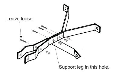
Assemble the bottom bracket the same way as the top with the addition of the support leg as shown. Place it between the brackets and secure it.
