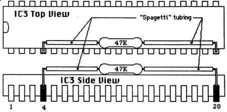
Solder the 47K ohm resistor directly to pins 4 and 20 of 1C3. Don't overheat or use too much solder. You must use an iron with voltage isolation on the tip!
