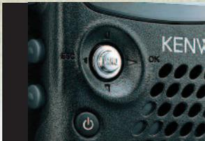
Vertical operation controls frequency, while horizontal movement controls band selection. There is also a 16-key pad with keys that are ergonomically spaced and illuminated for nighttime use.
