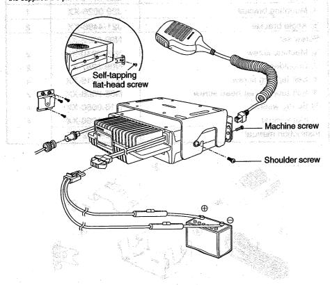
**IMPORTANT!** The transceiver operates in **12 V** negative ground systems only! Always check the battery polarity and voltage of the vehicle before installing the transceiver.
