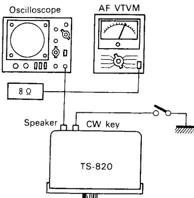
**Fig. 39 Adjustment of side tone**
