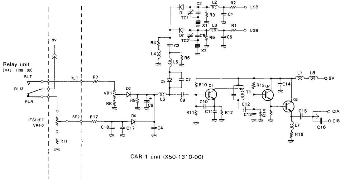
Fig. 9 IF SHIFT circuit
