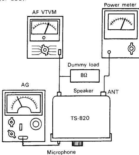
**Fig. 38 Adjustment of monitor level**
