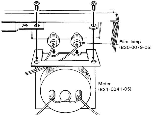
**Fig. 17(b) Removing the meter**
