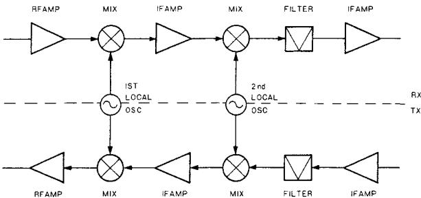
Fig. 1 Typical double conversion type
