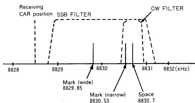
Fig. 10 RTTY frequency
