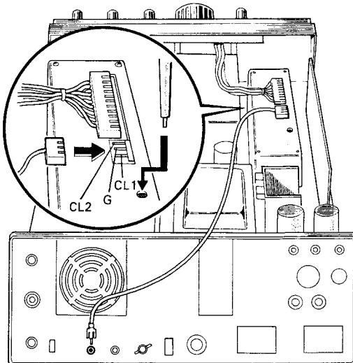
Fig. 32 Adjustment of counter standard oscillator frequency
