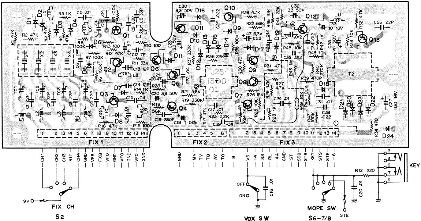
Q1: 2SK19(GR), Q2,3: 2SC460, Q4,5,7,8,10~12: 2SC733(Y), Q6,9: 2SA562(Y), Q13: 2SC735(Y), D1~4: 1S1587, D5,6: 1S658-2, D7,8,10,15,17: 1N60, D9,16,19~23: 1S1555, D18: WZ-130, D24: WZ-061
