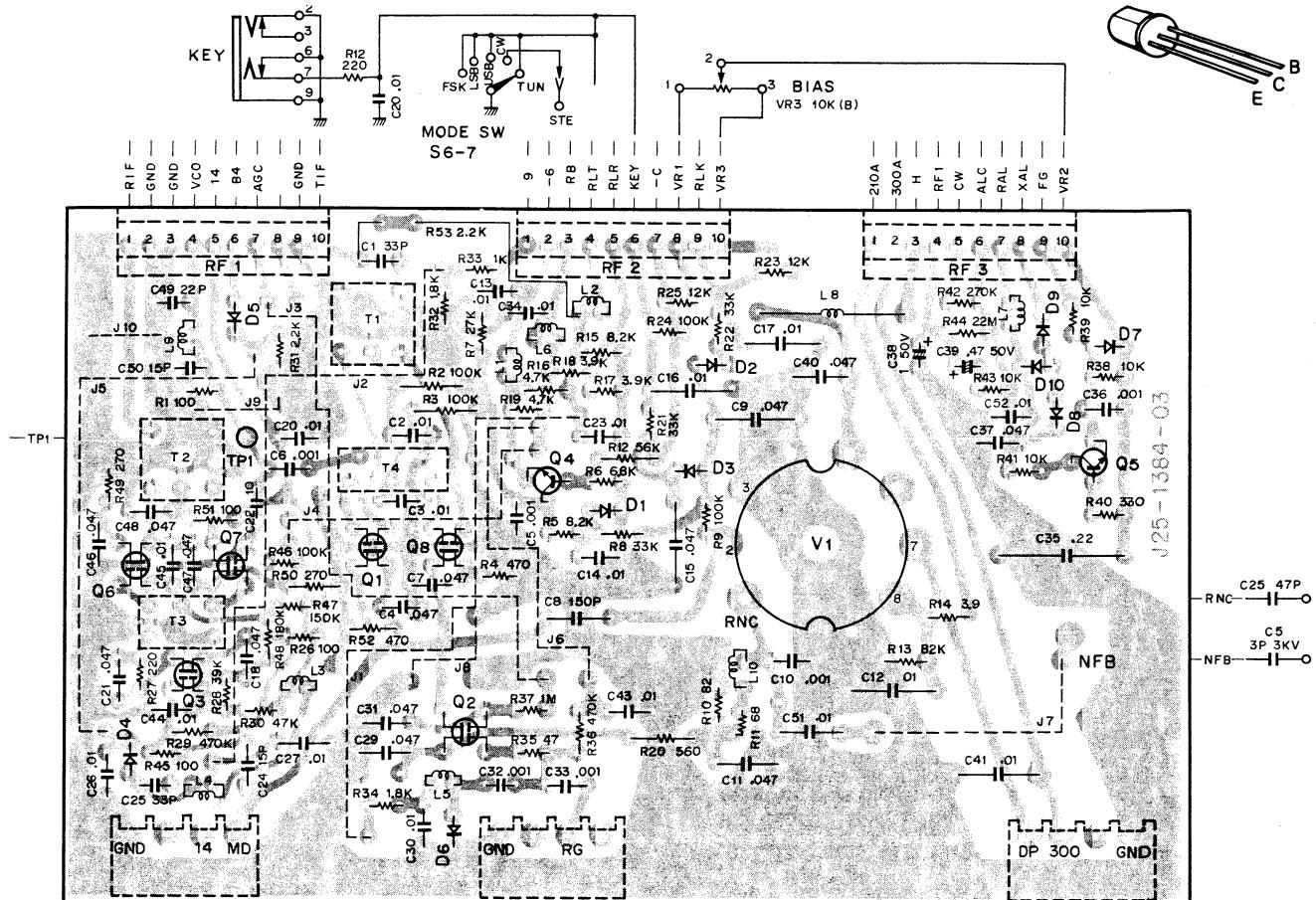
Q1,3,6~8: 3SK41(L), Q2: 3SK35(GR), Q4: 2SC733(Y), Q5: 2SC1515K(K), D1,8: WZ-090, D2,3,9,10: V06B, D4,6: 1S2588, D5,7: 1S1555, V1: 12BY7A
