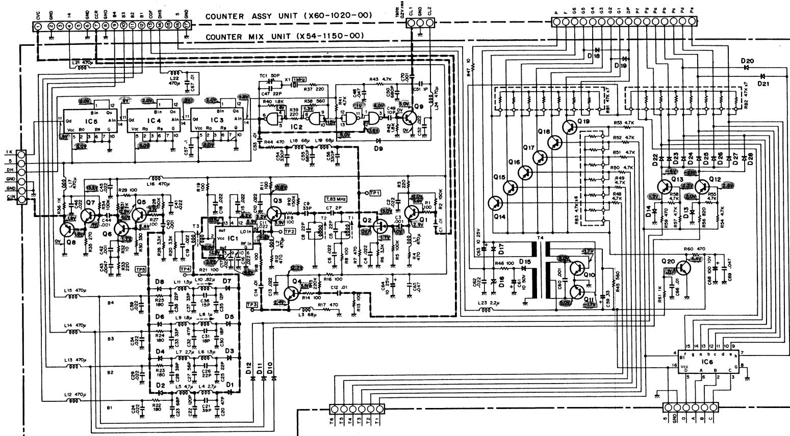
IC1: SN76514N, IC2: TD3400AP, IC3~5: TD3490BP, IC6:  $\mu$ PB249D, Q1,3~7,9: 2SC460(B), Q2: 3SK22(GR),
