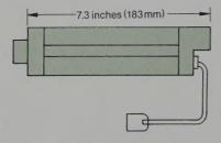
\* The depth of 7.3 inches (183mm) is the maximum effective length using flexible antenna cable/connector.
