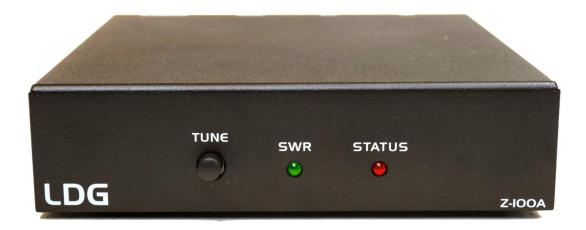
**TUNE Button:** Initiates either a memory tune or a full tune, and also toggles the tuner between "active" and "bypass" modes.
