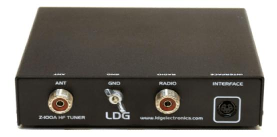
**ANT:** Connect the  $50\Omega$  coax antenna feedline to the standard SO-239 connector.
