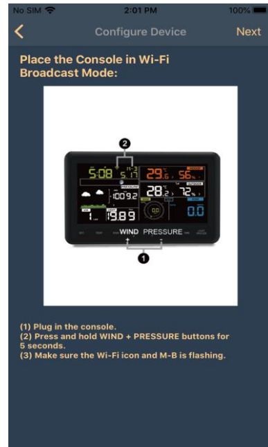
(c) Make sure the Wi-Fi icon is flashing rapidly. If not, press and hold the WIND+ and PRESSURE- buttons for four seconds. Tap Next .
