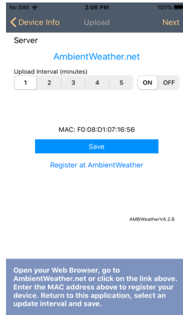
(i) Upload your data to AmbientWeather.net Select an upload interval in minutes and tap Save . Make a note of the MAC address. You will need this to create an account on AmbientWeather.net Tap Next .
