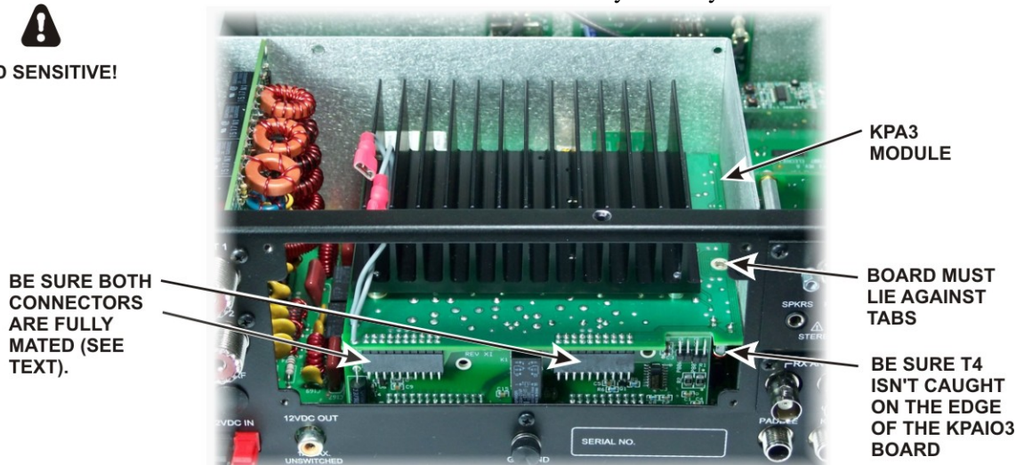
Figure 15. Mounting the KPA3 Module.
