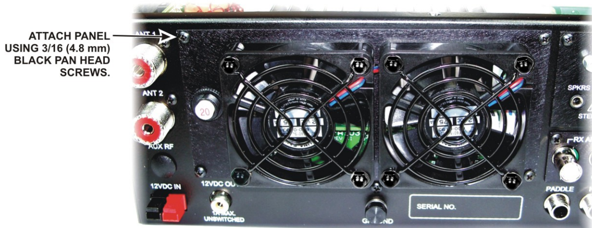
Figure 17. Fan Panel Installed on K3.
