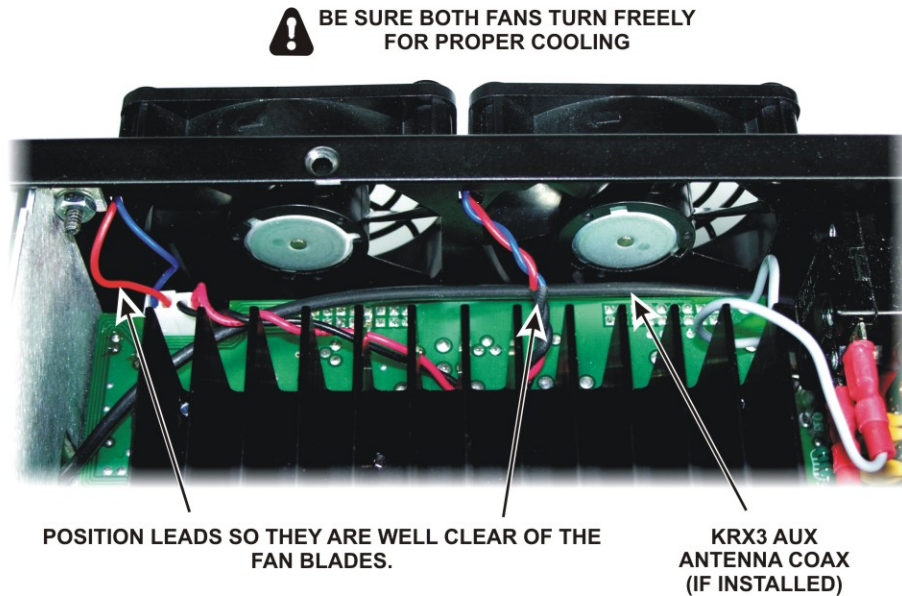
Figure 18. Positioning the Fan Leads.
