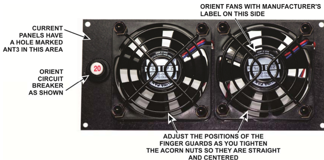
Figure 13, Completed Fan Panel from Rear.
