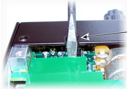
PLACE A SCREWDRIVER IN THE NOTCH PROVIDED AT EACH END OF THE FRONT PANEL SO IT PASSES AGAINST THE EDGE OF THE RF BOARD TO PRY THE FRONT PANEL ASSEMBLY LOOSE
