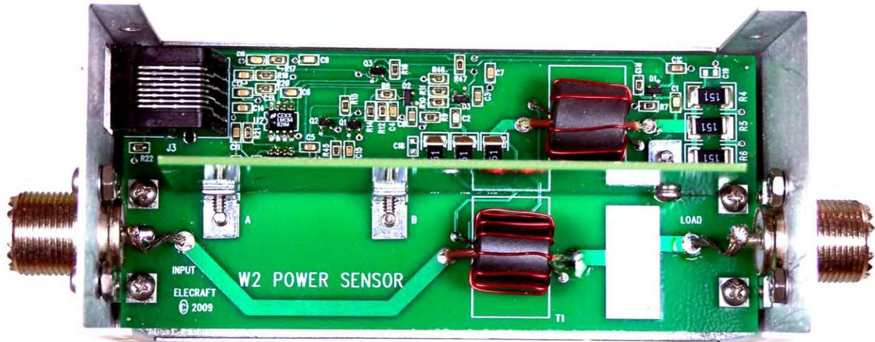
Figure 13. Typical Directional Coupler Sensor Interior View.
