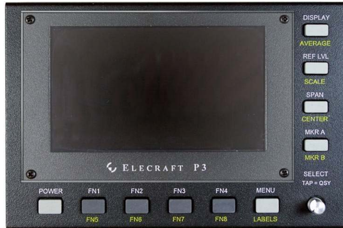
Figure 5. Bezel Mounted on Front Panel.
