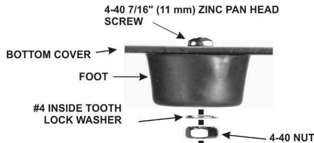
Figure 8. Installing Rear Feet.
