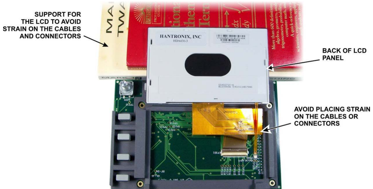
Figure 25. Removing LCD Panel from Rubber Key Matrix.
