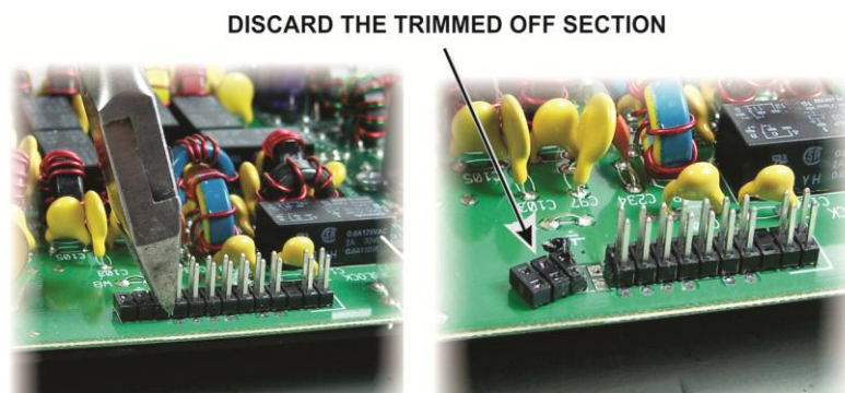
Figure 14. Cutting the Connector Housing.
