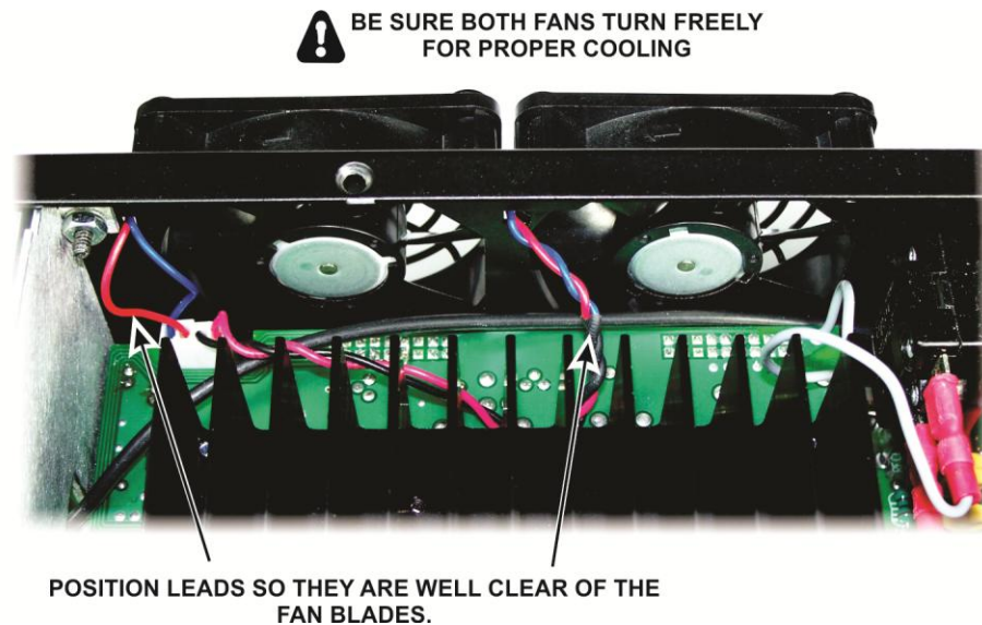
Figure 25. Positioning the Fan Leads.
