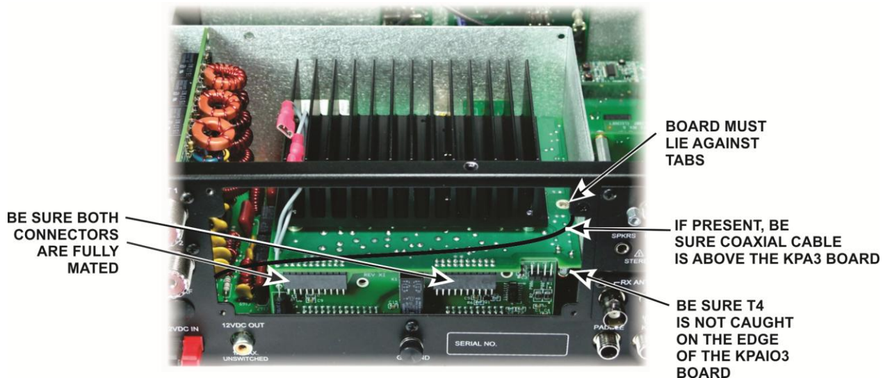
Figure 24. Reinstalling the KPA3 Module.
