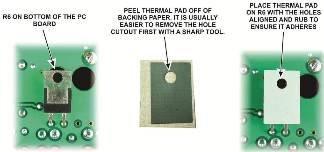
Figure 18. Placing Thermal Pad on R6.
