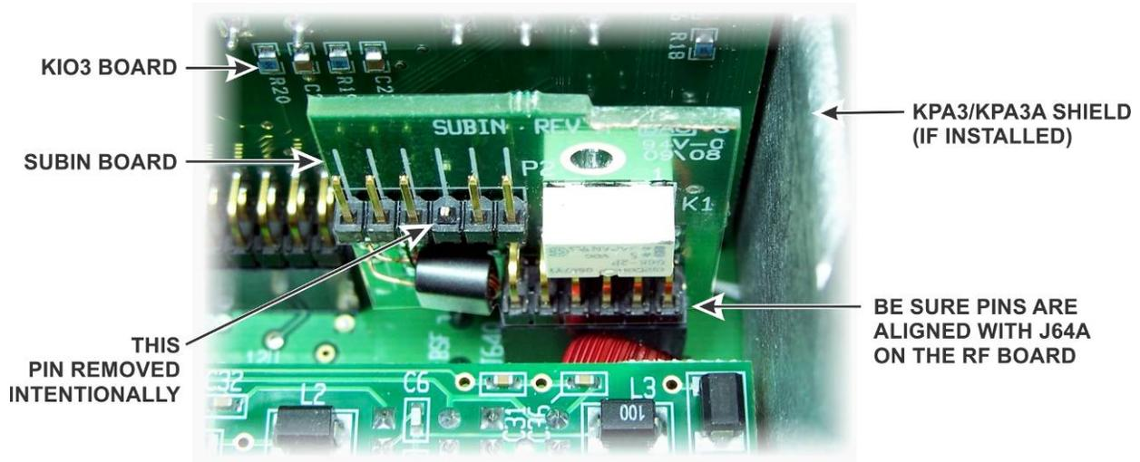
Figure 17. Replacing the SUBIN Board.
