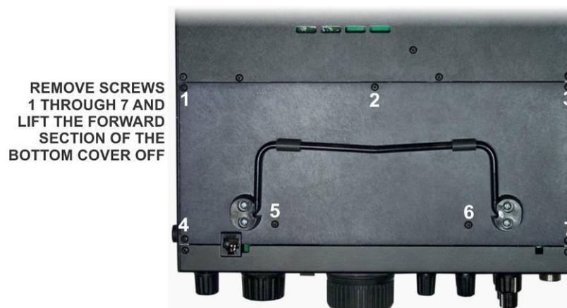
Figure 11. Removing Bottom Cover Front Section.
