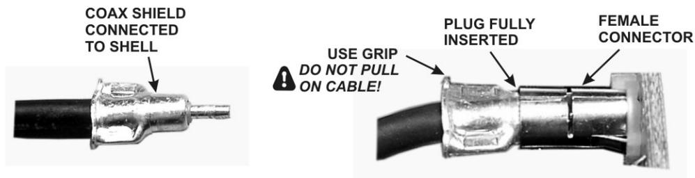
Figure 4. TMP Coaxial Connectors
