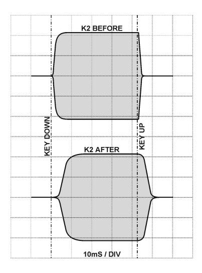
Most of the changes are in the key shaping circuitry (U10A, Control board). The R-C shaping network is reconfigured as a two-pole low-pass filter. In addition, a capacitor is added from the VPWR line (U8 pin 2) to ground to reduce the slew rate of the power-control DAC signal. Finally, a high-performance PIN diode replaces the original D36 on the RF board to prevent control signal leak-through during keying.
