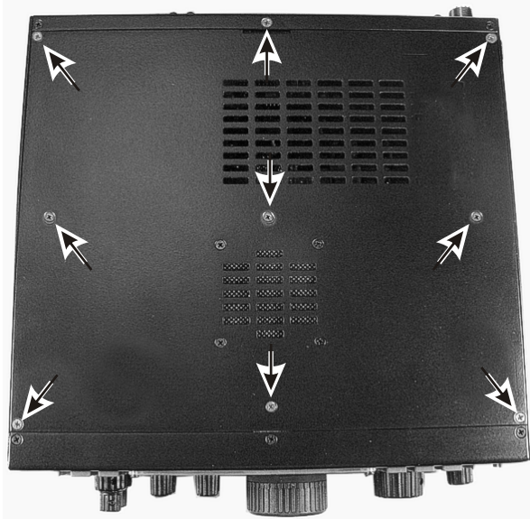
1 REMOVE SCREWS HOLDING TOP COVER.
