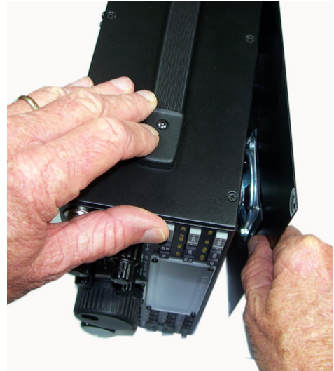
2 PLACE UNIT ON ITS SIDE FEET, THEN TIP FARTHER SO THE TOP COVER SWINGS OPEN FAR ENOUGH TO GRASP.
