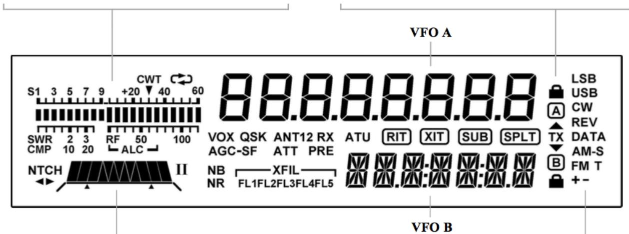
**Filter Passband Graphic:** Shows location of receive filter passband (pg. 12)
