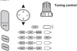
Each time you press the desired key, the Commander will automatically enter transmit mode and send the corresponding control command to the Transporter.
