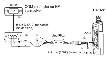
Attach the line filter to the cable.
