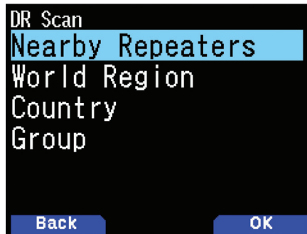
Figure 4 — If you're traveling, you can find nearby D-STAR repeaters based on your GPS location.
