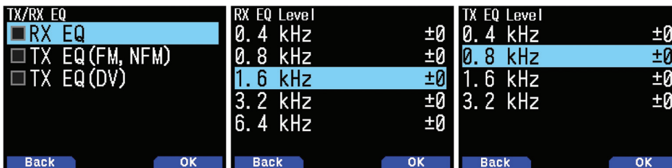
Figure 6 — Receive and transmit audio can be adjusted using the parametric equalizer menus.
