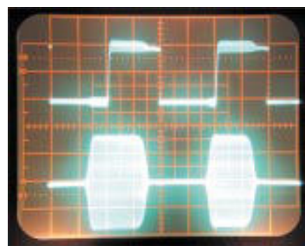
Figure 3—CW keying waveform for the TS-2000 showing the first two dits using external keying. Equivalent keying speed is 60 WPM. The upper trace is the actual key closure; the lower trace is the RF envelope. The transceiver was being operated at 100 W output at 14.02 MHz.
