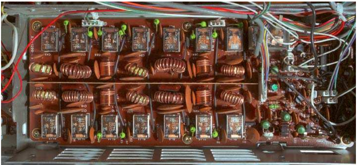
Relay-switched Low-pass filters used to remove harmonics from the transmitter output.
