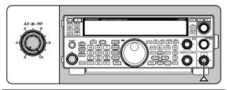
**Note:** The position of the **AF** control does not affect the volume of beeps caused by pressing keys nor the CW TX sidetone. The audio level for Digital mode operation is also independent of the **AF** control setting.
