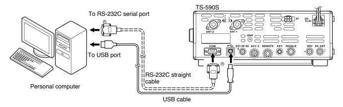
To transmit the signal from the PC, you must either turn the DATA VOX function ON or ground pin 9 (PKS) of the ACC2 connector to pin 8 (GND). (Refer to page 30 for the DATA VOX function.)
