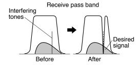
Press and hold **[BC (A.NOTCH)]** to toggle the Auto Notch Filter ON and OFF.
