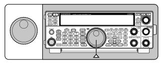
You may prefer directly entering a frequency using the numeric keypad if the desired frequency is far from the current frequency. Press **[ENT]**, then press the numeric keys as necessary. For details, refer to "Direct Frequency Entry" {page 28}.
