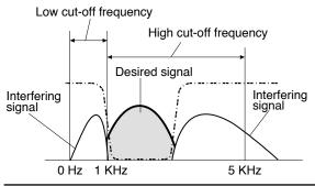
**Note:** The cut-off frequencies can be adjusted independently for each operating mode. When you change the operating mode, the previous setting is recalled for each operating mode.
