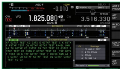
The CW decoder and bandscope screen.
