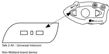
When successfully paired (no red/blue flashing light), open the intercom communication on the BTX1FM by following the instructions for “Manual activation;” on the other intercom press the phone redial button.
