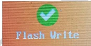
As soon as all data has been transferred from the CPS to the DB25-D, the text 'Flash Write' will disappear.
