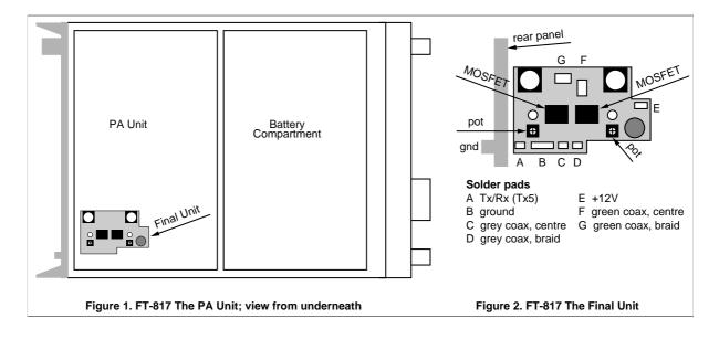
Remove the screw located in the centre of the lower cover by the edge of the battery compartment and then remove the 5 screws around the edge of the cover. Gently prise the cover away from the chassis.
