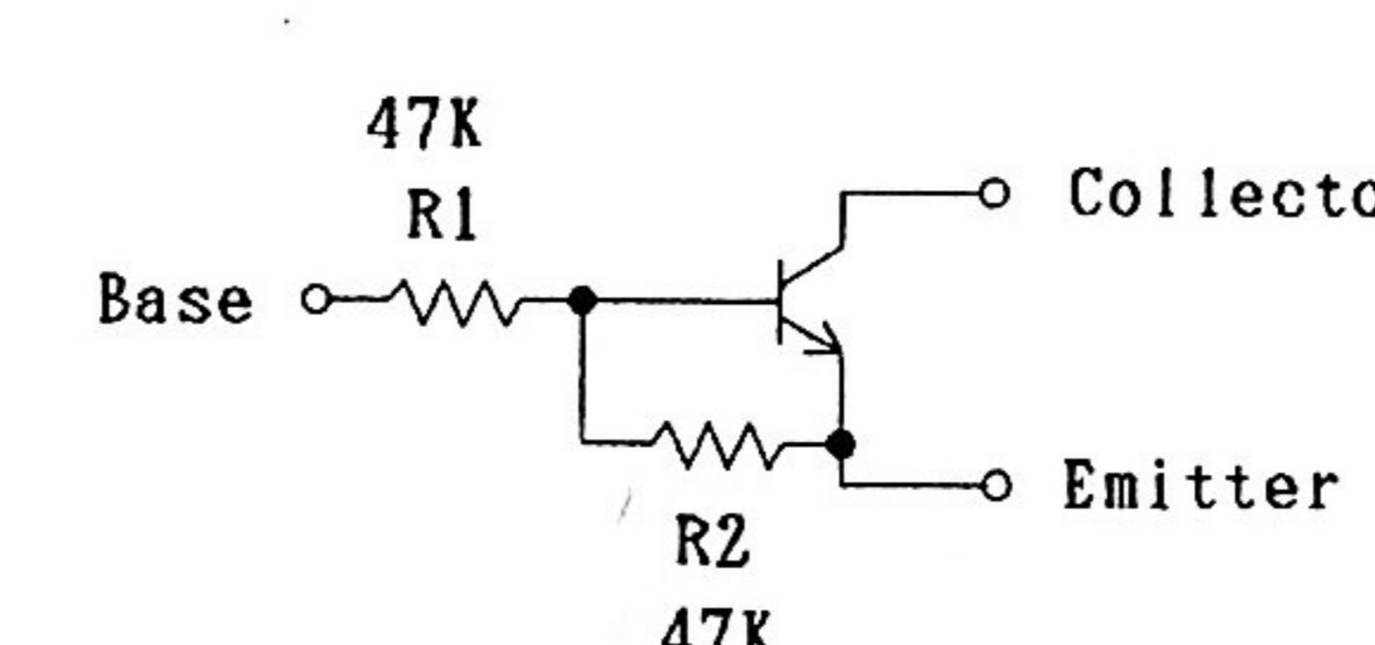
DTC144EK CIRCUIT DIAGRAM
