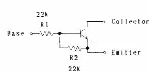
DTC124EK CIRCUIT DIAGRAM
