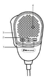
(1) UP and DOWN buttons These two buttons change the tuning channel. The first scrolls upwards through the tuned marine channels, the second scrolls downwards.
