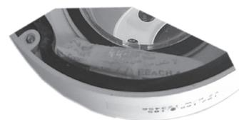
7. Reassemble the camera, sleeve, and ring. Position the assembly onto the base and adjust the camera to the correct viewing angle.
