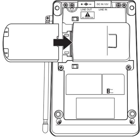
Make sure the BATTERY CHARGE LED lights. If the BATTERY CHARGE LED does not light, check to see that the AC Adapter is plugged in, and that the Battery Pack is seated into the Charging Compartment.
