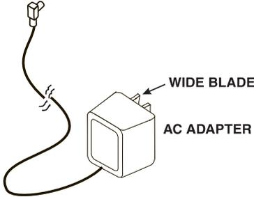
Do not alter the shape of the blades of the polarized plug.
