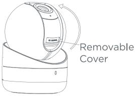
2 Open the cover to expose the memory card slot, and insert the memory card.
