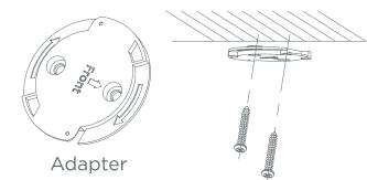
Fit the adapter into the camera bottom, and rotate the camera base clockwise to set it.
