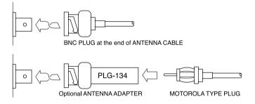
Connect your Antenna plug here. If you have a Motorola-type plug, use the optional adapter (PLG 134).
