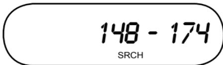
When **BAND** is pressed, this screen displays the band range to be searched. Press **BAND** again (or **UP/DOWN** within 3 seconds) to see other band ranges.
