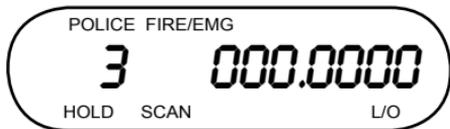
The screen cycles between two displays. The first screen shows that channel 3 on the **POLICE** bank (40.0600) is selected and the second screen shows that the null frequency (000.0000) is ready to be programmed.
