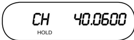
From a normal scan setting (a channel bank is flashing), press **PROG**. HOLD displays and **CH** displays and flashes. Press and hold **L/O** for 2.5 seconds.
