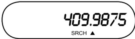
This SEARCH screen shows that frequency 409.9875 has been found through an upward search. Pointers (▲ or ▼) indicate the direction of the search - up or down.
