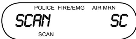
This screen shows BC355C is actively scanning a displayed bank. "SCAN" scrolls from right to left across the screen, and the scanned bank will flash.
