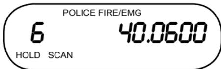
Press **PROG**. The scanner programs the frequency into the indicated channel and then goes into SCAN HOLD mode.
