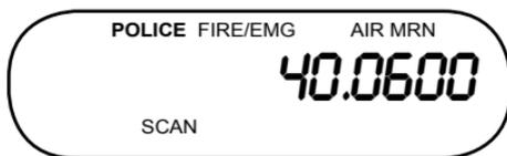
This SCAN screen shows that frequency 40.0600 has been found through a search of the active (flashing) POLICE bank.
