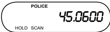
This screen shows that the scanner has been put on HOLD to monitor frequency 45.0600 on the Police bank.
