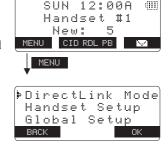
In the submenu, *volume*/ ▲ or ▼ is used to select an item. Press the **OK** soft key to confirm your selection. To return to the previous screen, press the **BACK** soft key. For detailed instructions, see the following sections for the desired submenu.
