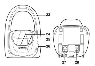
23.Base Antenna 24.Base Charging Contacts 25.**Charge** LED 26.*Find handset* Key (P. 34) 27.**TEL LINE** Jack 28.**DC IN 9V** Jack
