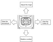
You will also use the joystick to make menu selections. Highlight the option you want by moving the joystick up, down, right, or left. This will move the cursor; the option currently highlighted appears in reversed out text:
