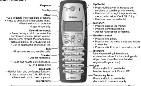
Note: Each handset can be turned off to conserve battery life. To turn off the handset, press and hold (m). When the handset is turned off, you cannot make or receive calls on that handset. To turn the handset on again, press and hold (m) or place the handset in the charger.
