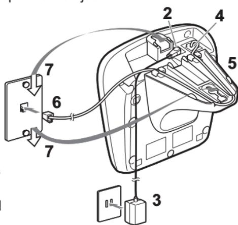
**Note:** To mount the phone directly on the wall, insert two 1 3/8 inch, #10 screws (not supplied) into the wall using anchors suitable for the wall material. Place the screws 3 15/16 inches apart, and allow 1/8 inch free space between the wall and screw heads.
