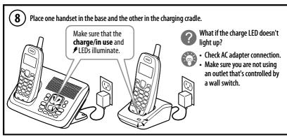
Note: For optimum battery life, charge all of your handsets completely before you connect the telephone cord. The first time you charge a new battery, allow 15 to 20 hours.
