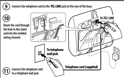
Note: If the telephone cord does not fit into your telephone wall jack, contact your local phone provider for assistance.
