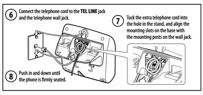
Note: To mount the phone directly on the wall, insert two 1 3/8 inch, #10 screws (not supplied) into the wall using anchors suitable for the wall material. Place the screws 3 15/16 inches apart, and allow 1/8 inch free space between the wall and screw heads.
